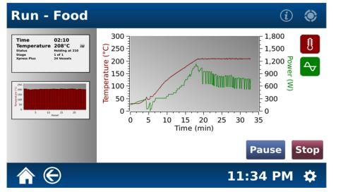
*Figure 3. Temperature and Power Graph from MARS 6*
