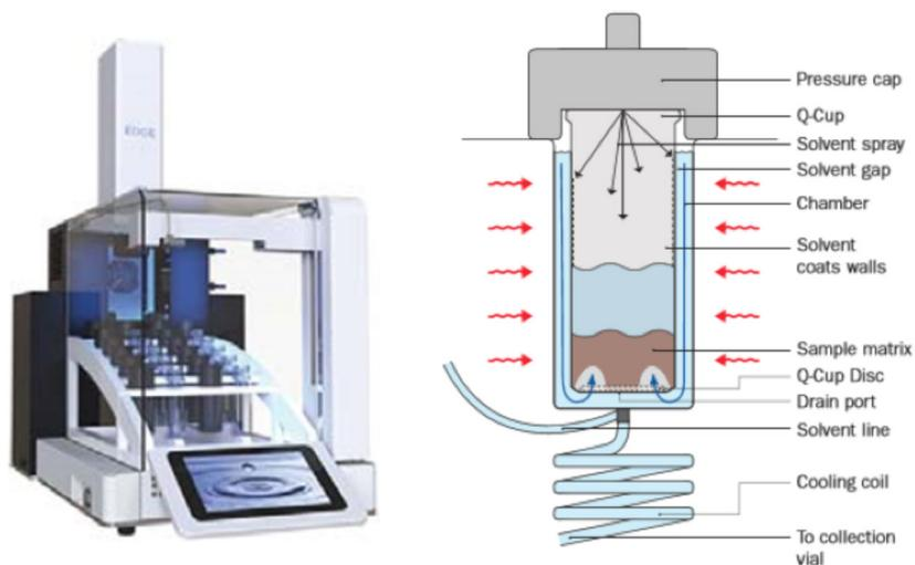
**Q-Cup Technology combines the processes of Pressurized Fluid Extraction and Dispersive Solid Phase Extraction into one instrument.**
